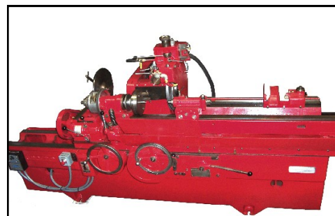
APT Van Norman 253 cam grinder. Basically a "copying" machine, the "smart" part is the master that it copies from, and hopefully the operator!
